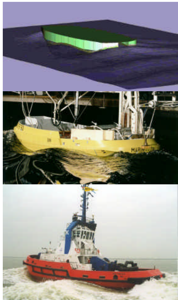
Figure 6: Comparison of wave patterns in three different stages: calculations, model scale, full scale
